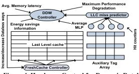
Figure 4. Hardware Control for Dynamic Dataless Ways (DDW). Additions are shaded.
