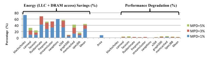
Figure 5. Energy/area savings and performance degradation with FreshCache.
